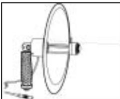
Select the parabolic sensor if the leaks you are detecting are outside the range of the EDS (Fig 3). The parabolic shape focuses faint ultrasonic waves onto a super sensitive ultrasonic crystal amplifying and thereby extending the detection range by up to 250'. The laser sight pinpoints the exact source of the leakage, or use the rifle sight in bright daylight.
