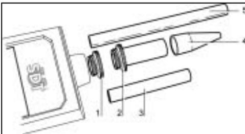
All SDT 170 ultrasonic detectors are equipped with an internal airborne sensor for detection of pressure and vacuum leaks. This sensor is ideal for day to day leak detection where the source of the leak is within reach of the inspector. Use in conjunction with the precision indicator kit (shown in Fig 1) to pinpoint the exact source of leakage.
